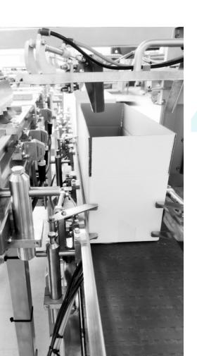
Specially designed deflector utilizes an advanced sensor system and vision technology to ensure precise **quality control**, preventing the inclusion of unwanted boxes during the packaging process.
